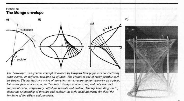
c) Model built by Beltrami showing a Monge envelope in three dimensions. The very obvious curve of the sides of the figure does not physically exist, but is formed as the result of the series of straight strings.
