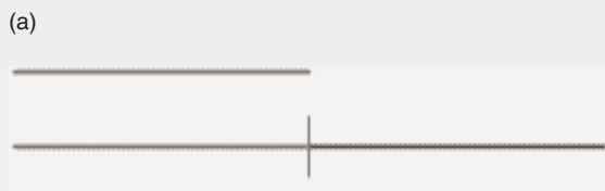
FIGURE 1. Doubling and "powers." (a) The magnitude which has the "power" to double the length of a line is produced by simple extension. (b) The magnitude which has the power to produce a square of double area, is the diagonal of the smaller square, and is called "the geometric mean" between the two squares. The magnitude of diagonal BC is incommensurable with, and cannot be produced by, the magnitude of side AB of the smaller square. (c) The magnitude which has the power to produce a cube of double volume, is different from the magnitudes which have the power to double a square, or a line. It is the smaller of two geometric means between the two cubes. This magnitude is incommensurable with both lower magnitudes, the square and the line.
